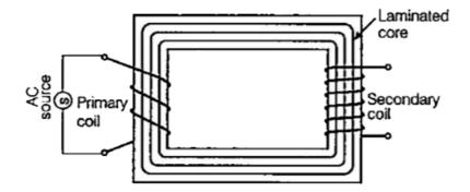
Working and Principle The value of the emf depends on the number of turns in the secodary. We consider an ideal transformer in which the primary coil has negligble resistane and all the flux in the core links both primary and secondary windings. Let  $\phi$  be the flux in each turn in the core at time t due
