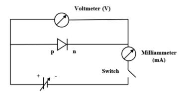
The circuit arrangement for studying V-I characteristics of a p-n junction diode in reverse bias is given below.
