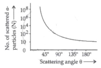
The strongly repulsive force exerted by the positively charged nucleus causes the scattering of  $\alpha$ -particles at  $\theta > 90^{\circ}$ . Because the nucleus is so small, there are fewer distributed  $\alpha$ -particles.
