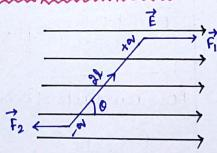
0 is the angle between dipole moment and intensity.
