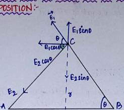
C is any point en the equitorial line at a distance of from the centre of the dipole
