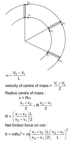
$$fr = \frac{m(v_2 - v_1)(v_1 + v_2)}{2L} = \frac{m(v_2^2 - v_1^2)}{2L}$$
