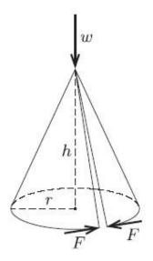
The cone is placed on a horizontal, frictionless table-top, and loaded at its apex with a vertical force of magnitude w, without collapsing. The splaying of the cone is opposed by a pair of forces of magnitude F acting tangentially at the join in the base circle (see figure). Ignoring any frictional or bending effects in
